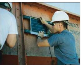
Photos: (Top) By using the Solargizer Solar Charger and solenoid-controlled valves on its radio-controlled ballast cars, CSXT eliminated the use of one locomotive per unit train due to the reduced volume of air required. This alone will provide considerable savings every year. (Bottom) The Solargizer Solar Charger is so effective in increasing battery performance and reducing battery related costs, CSXT installed units on hundreds of radio-controlled ballast cars.
